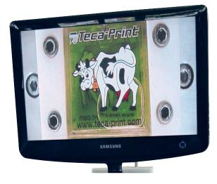
The operator can act immediately even before drying is completed and adjust the printing process. The LCD monitor shows an enlarged view of the actual printed image and can be located up to 5 m from the camera.
